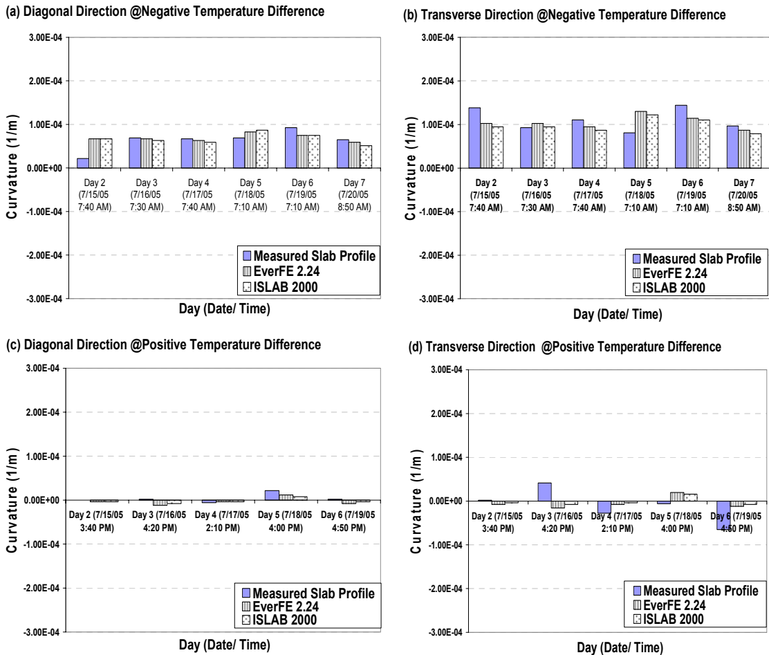
Figure 5-14 Comparisons of curvature ( k ) between measured and FE-predicted slab curvature profiles using method 2 in test section 1:(a) diagonal direction at negative temperature difference condition; (b) transverse direction at negative temperature difference condition; (c) diagonal direction at positive temperature difference condition; (d) transverse direction at positive temperature difference condition
