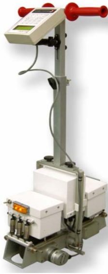
Figure 3-8 ICC Rollingprofiler (SurPRO 2000 ® ) (adopted from ICC., 2006)
