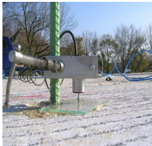
Figure 3-7 Typical LVDT installation in this study
