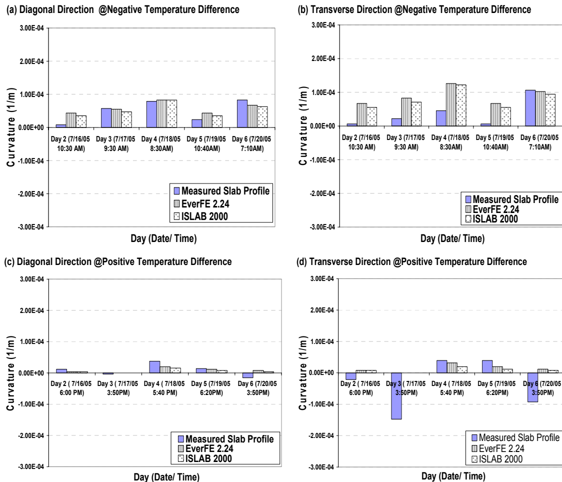
Figure 5-15 Comparisons of curvature ( k ) between measured and FE-predicted slab curvature profiles using method 2 in test section 2:(a) diagonal direction at negative temperature difference condition; (b) transverse direction at negative temperature difference condition; (c) diagonal direction at positive temperature difference condition; (d) transverse direction at positive temperature difference condition
